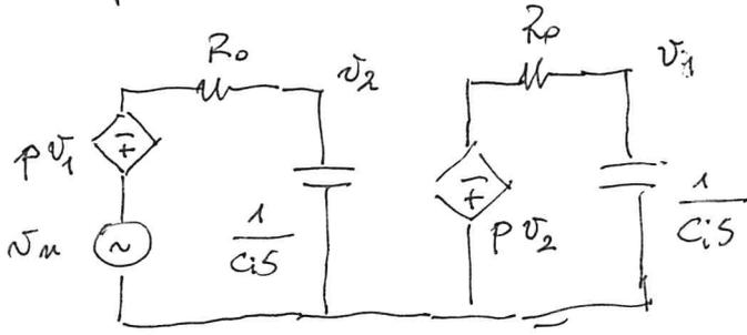
$$V_1 = -pV_2 \frac{1}{R_0 C_i S + 1}$$
