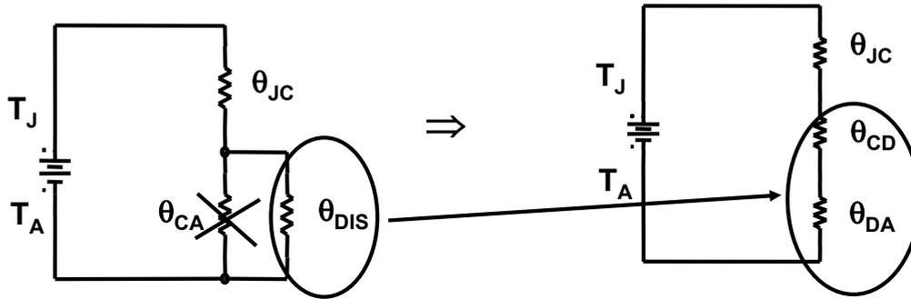
$$\Delta T = \Theta \cdot P_D \quad \theta_{JC} = \frac{200 - 25}{150} = 1.17 \text{ } ^\circ\text{C/W} \quad \theta_{CD} = 0.1 \div 0.4 \text{ } ^\circ\text{C/W}$$
