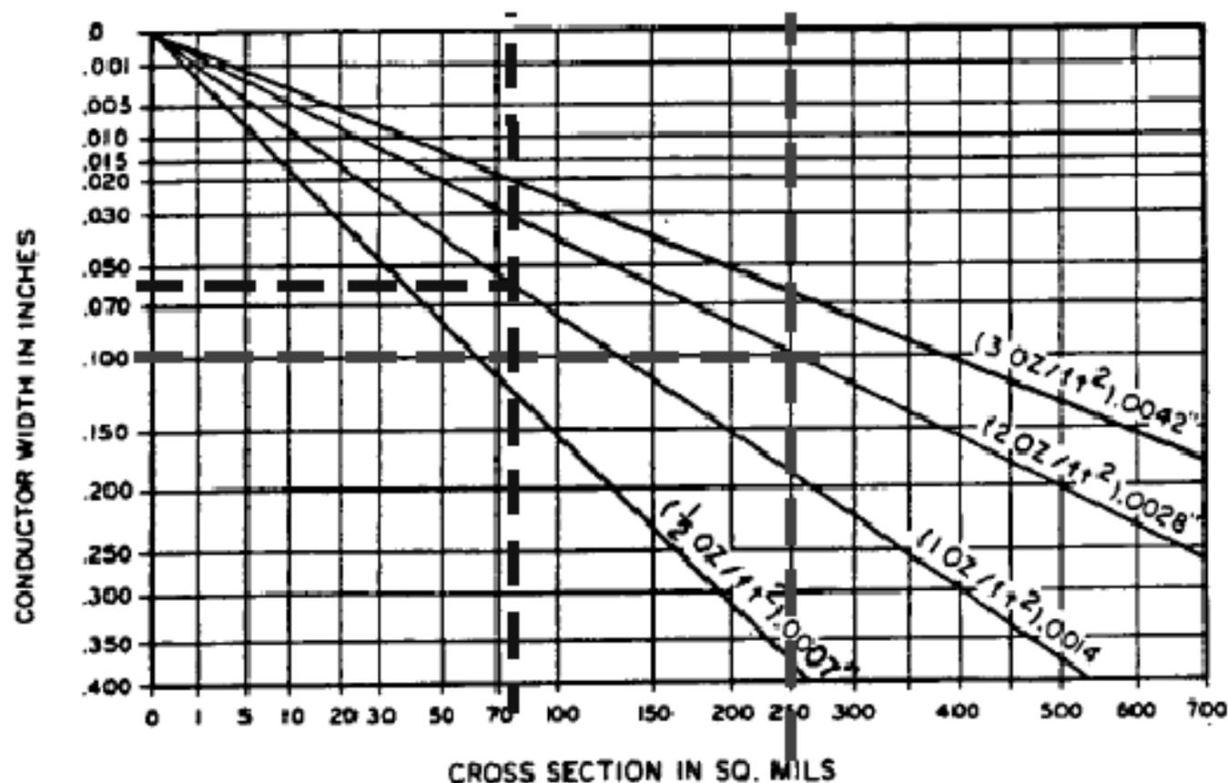
Figure B Conductor width to cross-section relationship
