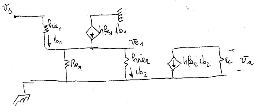
$$V_s = hfe_1 i_b_1 + (R_{e1} \parallel R_{e2}) (hfe_1 + 1) i_b_1$$
