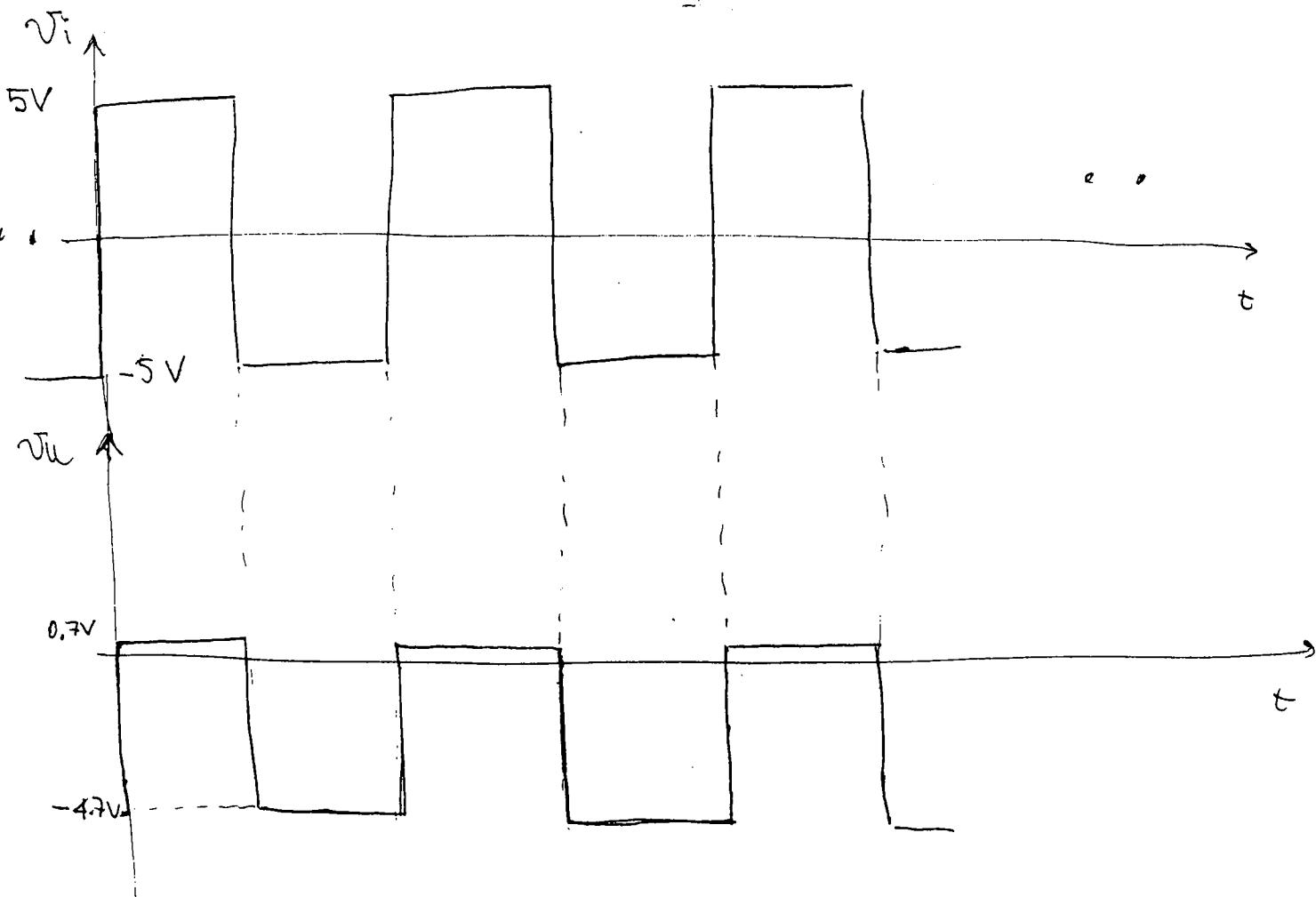
$$V_u = \frac{1}{T} \int_T V_u(t) dt = \frac{1}{T} \left( 0.7 \cdot \frac{T}{2} - 4.7 \cdot \frac{T}{2} \right) V = -2V$$
