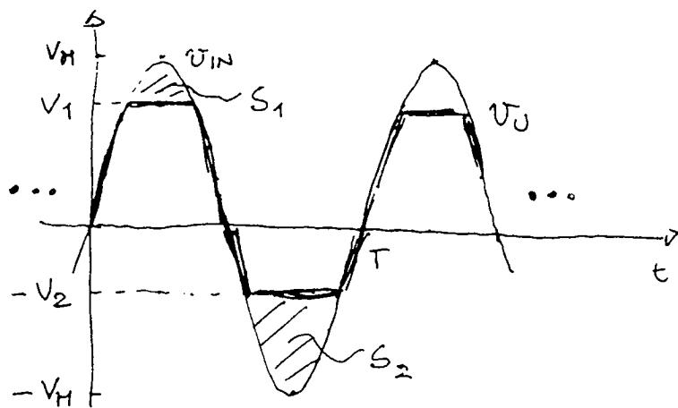
$$V_1 = V_F + V_{Z2} = 7V$$
