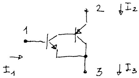
$$\begin{cases} I_2 = I_1 \cdot h_{FE1} (h_{FE2} + 1) = I_1 \cdot h^* \\ I_3 = I_1 + I_2 = I_1 (h^* + 1) \end{cases}$$
