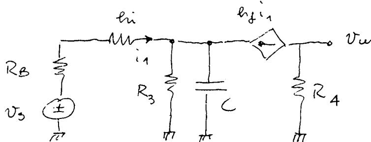
$$R_B = R_1 \parallel R_2 = 11,67k\Omega$$
