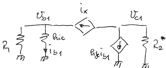
$$R_2^* = \frac{R_2 + h_{ie}}{h_{fe} + 1} = 502 \Omega$$
