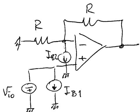
$$V_{uo} = -2V_{io} + RI_{B2} =$$
