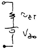
$$V_{z0} = V_{zT} - I_{zT} r_{zT} = 5.8V$$
