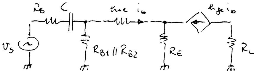
$$h_{ie} = \frac{V_T}{I_C} h_{FE} + r_{bb'} \approx 520 \Omega$$
