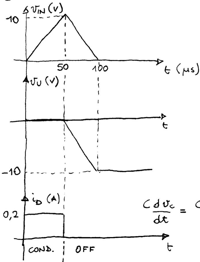
$$C \frac{dV_C}{dt} = C \frac{dV_{IN}}{dt} = 1\mu \cdot \frac{10}{50\mu} = 0.2 \text{ A}$$
