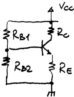
$$I_B = \frac{V_B - V_{BE0}}{R_B + (h_{FE} + 1) R_E} = 24,92 \mu\text{A}$$
