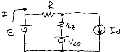
$$r_z = 1 \Omega \quad V_{z0} = 14,9 \text{ V}$$
