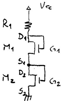
$$\left. \begin{aligned} V_{GD1} &= \phi \\ V_{GD2} &= \phi \end{aligned} \right\} M_1 \text{ e } M_2 \text{ saturi}$$
