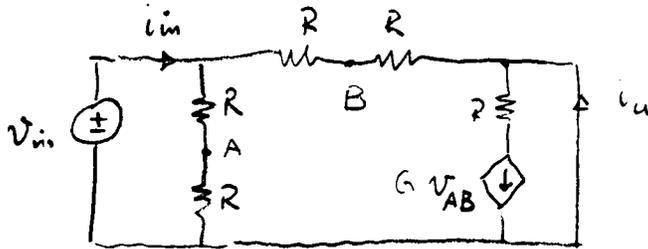
Si ha  $v_{AB} = \frac{v_{in}}{2} - \frac{v_{in}}{2} = 0$ . Quindi
