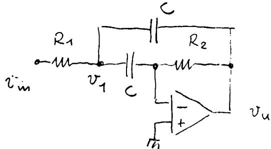
$$v_u = -v_1 R_2 C s \quad (\text{derivatore})$$
