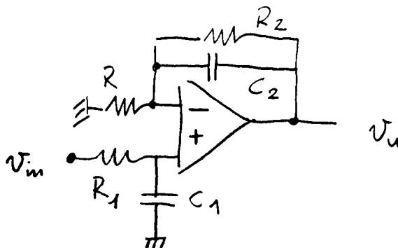
$$\begin{aligned} R_1 &= 10 \text{ k}\Omega \\ C_1 &= 100 \text{ nF} \\ R_2 &= 100 \text{ k}\Omega \\ C_2 &= 10 \text{ mF} \\ R &= 1 \text{ k}\Omega \end{aligned}$$
