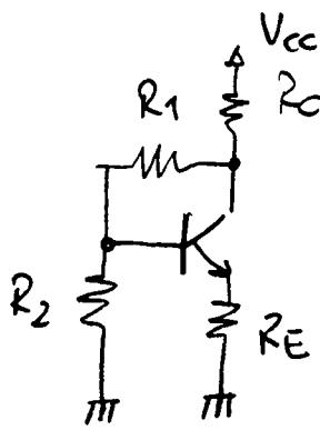
$$\begin{aligned} V_{cc} &= 12 \text{ V} \\ R_c &= 1 \text{ k}\Omega \\ R_E &= 100 \Omega \\ R_1 &= 190 \text{ k}\Omega \\ R_2 &= 120 \text{ k}\Omega \\ h_{FE} &= h_{fE} = 249 \\ r_{bb'} &= 200 \Omega \end{aligned}$$
