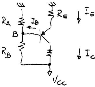
$$V_{BB} = V_{cc} \frac{R_A}{R_A + R_B} = -4V ; \quad R_{eq} = R_A \parallel R_B = 2.93 k\Omega$$
