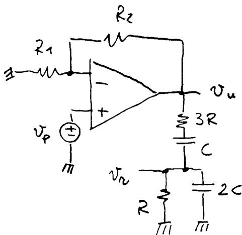
$$bA = \frac{V_u}{V_p} = \left(1 + \frac{R_2}{R_1}\right) \cdot \frac{\frac{R}{2RCS+1}}{\frac{R}{2RCS+1} + 3R + \frac{1}{CS}} = \left(1 + \frac{R_2}{R_1}\right) \cdot \frac{RCS}{6RCS + 6(RCS)^2 + 1}$$
