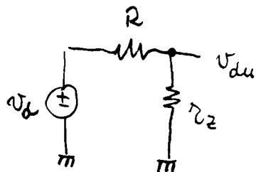
$$\frac{V_{du}}{V_d} = \frac{r_z}{R + r_z} = 0,0904$$
