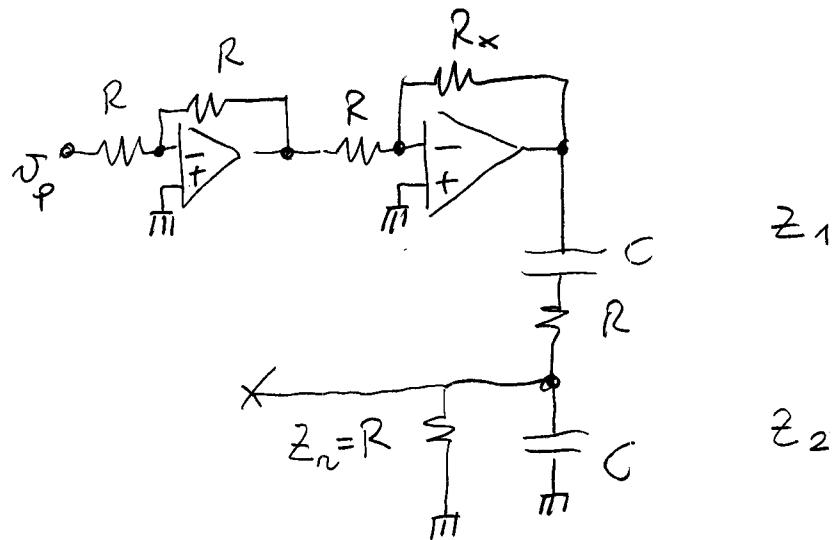
$$bA = \frac{R_x}{R} \cdot \frac{Z_2}{Z_1 + Z_2} = \frac{R_x}{R_0} \cdot \frac{\frac{j\omega RC}{(1 - \omega^2 RC) + 3j\omega RC}}{1}$$
