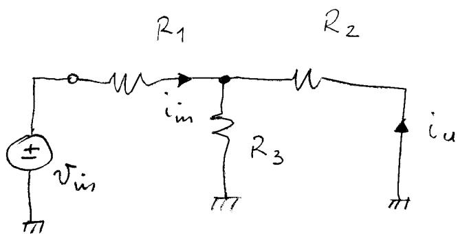
$$g_i = \left. \frac{i_{in}}{V_{in}} \right|_{V_u=0} = \frac{1}{R_1 + R_2 // R_3} = \frac{R_2 + R_3}{R_1 R_2 + R_1 R_3 + R_2 R_3}$$
