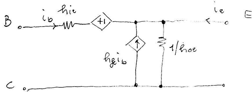
$$h_{fe} = \frac{i_e}{i_b} \Big|_{V_{ce}=0}$$
