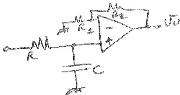
$$A_V(s) = \left(1 + \frac{R_2}{R_1}\right) \frac{1}{\frac{s}{\omega_p} + 1}$$
