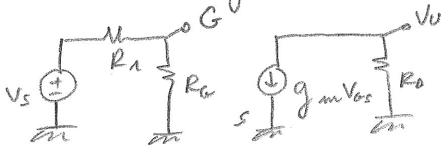
$$A_\infty = -\frac{R_o g_m R_f}{R_f + R_1} = 3,091 \quad (19,17 \text{ dB})$$
