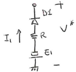
D1 conduce se:  $I_1 > 0 \rightarrow -V^* - V_{D1} - E_1 > 0$
