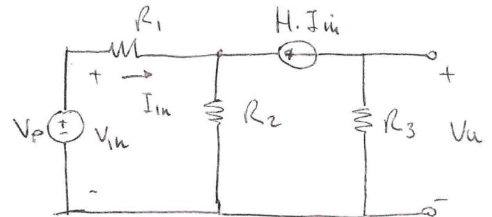
$$V_u = - \frac{R_3 H}{R_1 + R_2(1+H)} \cdot V_p$$
