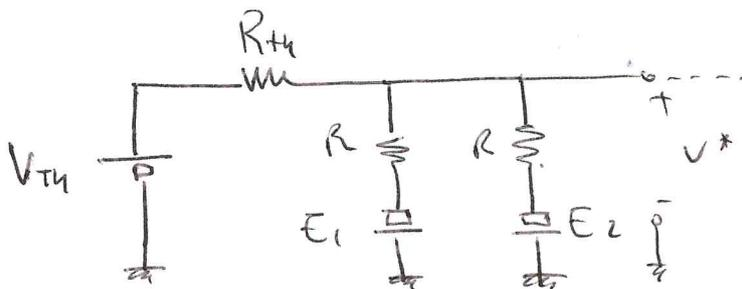
$$V^* = V_{TH} \cdot \frac{R/2}{R_{TH} + R/2} - E_1 \cdot \frac{R_{TH} \parallel R}{R + R_{TH} \parallel R} - E_2 \cdot \frac{R_{TH} \parallel R}{R + R_{TH} \parallel R}$$
