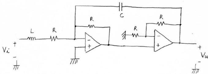
$R = 5 \text{ k}\Omega$  ,  $C = 10 \text{ nF}$  ,  $L = 10 \text{ nH}$  ;
