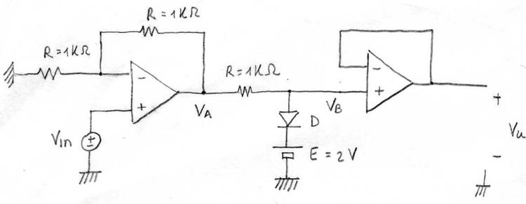
$$V_A = V_{in} \left( 1 + \frac{R}{R} \right) = 2 V_{in}$$
