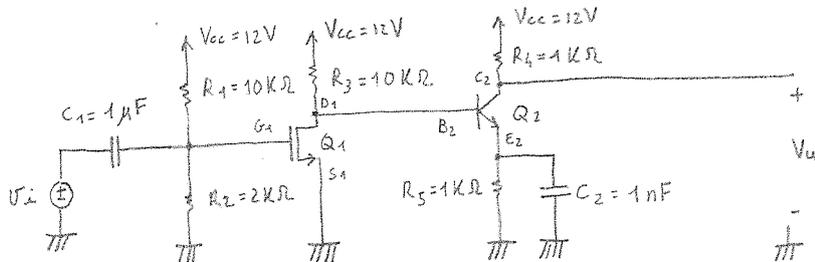
$$K = \mu_n C_{ox} \frac{W}{L} = 2 \frac{\text{mA}}{\text{V}^2}$$
