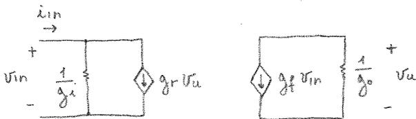
$$V_u = -g_f V_{in} \cdot \frac{1}{g_o} \rightarrow f_f = \frac{V_u}{V_{in}} \Big|_{i_u=0} = -\frac{g_f}{g_o}$$
