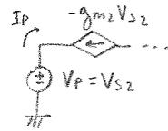
$$R_V = \frac{V_p}{I_p} = \frac{V_{S2}}{g_{m2}V_{S2}} = \frac{1}{g_{m2}}$$
