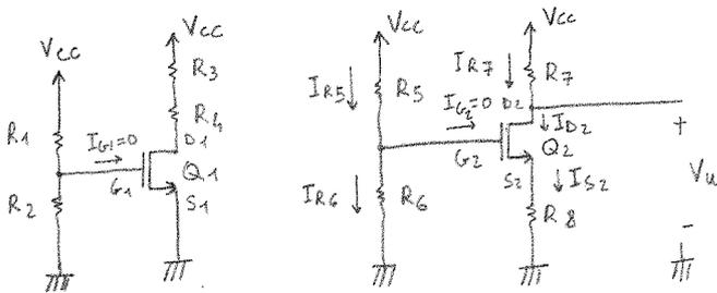
$$I_{R_7} = \frac{V_{cc} - V_u}{R_7} = 2\text{mA} = I_{D_2} = I_{S_2}$$
