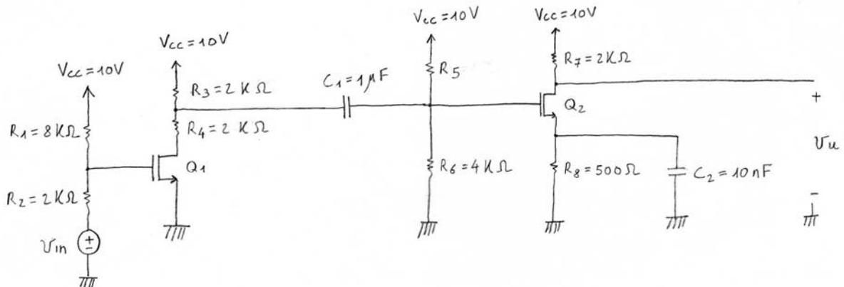
PER  $Q_1$ :  $\frac{1}{2} \mu\text{n Cox} \frac{W_1}{L_1} = 1 \frac{\text{mA}}{\text{V}^2}$
