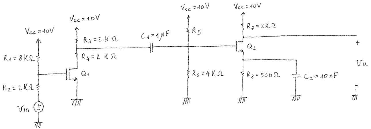
$$\text{PER } Q_1: \frac{1}{2} \mu_n C_{ox} \frac{W_1}{L_1} = 1 \frac{\text{mA}}{\text{V}^2}$$
