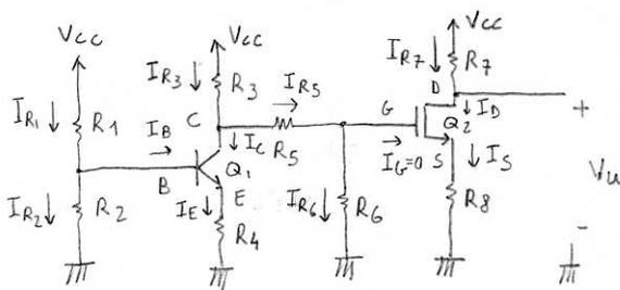
$$I_{R7} = \frac{V_{cc} - V_u}{R_7} = 2 \text{ mA} = I_D = I_S$$
