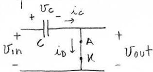
quindi  $v_{out} = 0$ ,  $V_C = V_{in} - V_{out} = V_{in}$ ;
