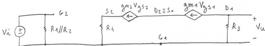
$$V_u = -R_3 g_{m1} V_{gs1}$$
