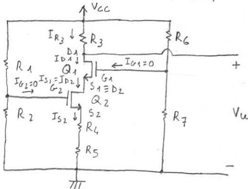
$$V_{G2} = V_{cc} \frac{R_2}{R_1 + R_2} = 4V$$
