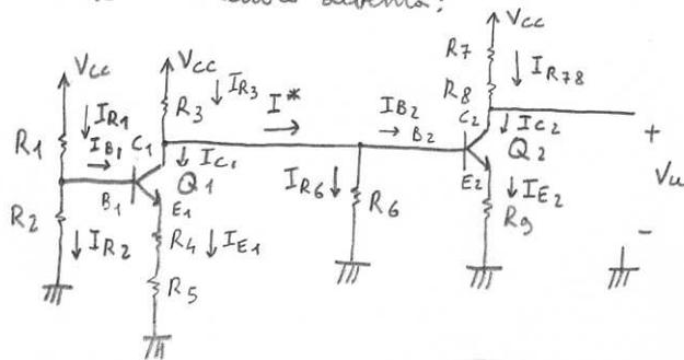
$$I_{R78} = \frac{V_{CC} - V_u}{R_7 + R_8} = 2 \text{ mA} = I_{C2}$$
