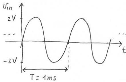
$$v_{in} = V_M \sin(\omega t) \quad \text{con} \quad V_M = 2V, \quad \omega = \frac{2\pi}{T}, \quad T = 1ms$$
