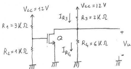
$$\text{per } Q: \quad \frac{1}{2} \mu_n C_{ox} \frac{W}{L} = 1 \frac{\text{mA}}{\text{V}^2}$$
