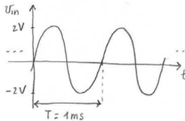
$$v_{in} = V_M \sin(\omega t) \quad \text{con} \quad V_M = 2V, \quad \omega = \frac{2\pi}{T}, \quad T = 1ms$$
