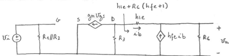
$$v_u = R_6 (h_{fe} + 1) i_b$$
