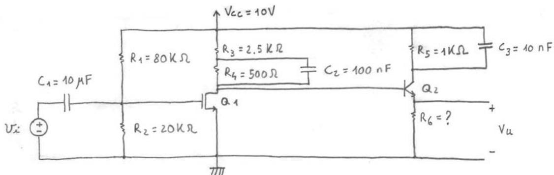
per  $Q_1$ :  $V_T = 1V$ ,  $\frac{1}{2} \mu_n C_{ox} \frac{W}{L} = \frac{2mA}{V^2}$
