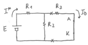
$$I^* = \frac{E}{R_1 + R_2 // R_3} = 2.25 \text{ mA}$$
