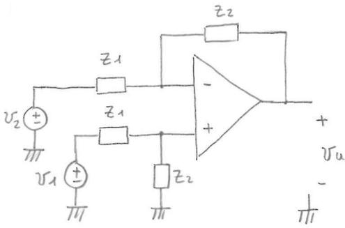
$$v_u = \left( v_1 \frac{z_2}{z_1 + z_2} \right) \left( 1 + \frac{z_2}{z_1} \right) + v_2 \left( -\frac{z_2}{z_1} \right) = \frac{z_2}{z_1} (v_1 - v_2)$$
