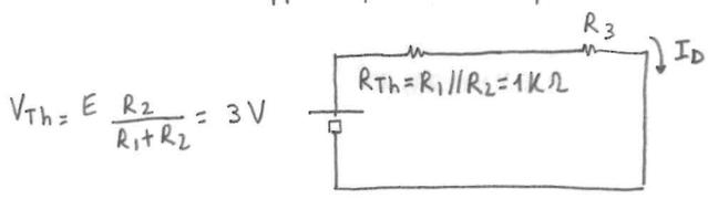
$$I_D = \frac{V_{Th}}{R_{Th} + R_3} = 1.5 \text{ mA}$$
