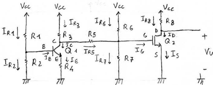
$$I_{R8} = \frac{V_{CC} - V_u}{R_8} = 2 \text{ mA} = I_D = I_S$$
