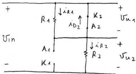
$$i_{R2} = \frac{V_{in}}{R_2} < 0 \quad (\text{essendo } V_{in} < 0)$$
