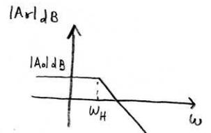
con  $A_0 = 1 + \frac{R_3}{R_2} = 3 \rightarrow R_3 = 2R_2$ , ad es  $R_2 = 1 \text{ K}\Omega$ ,  $R_3 = 2 \text{ K}\Omega$
