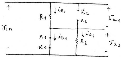
$$i_{R1} = \frac{V_{in}}{R_1} > 0 \quad (\text{essendo } V_{in} > 0)$$
