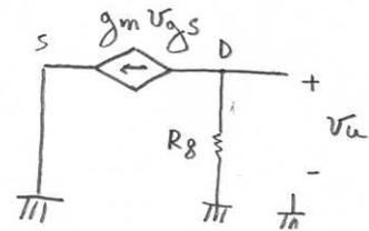
$$V_u = -R_8 g_m V_{gs}$$
