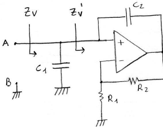
$$\begin{aligned} C_1 &= 500 \text{ nF} \\ C_2 &= 100 \text{ nF} \\ R_1 &= 1 \text{ K}\Omega \\ R_2 &= 2 \text{ K}\Omega \end{aligned}$$
