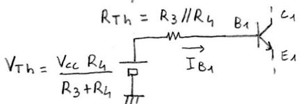
$$\text{con } V_{Th} = V_{cc} \frac{R_4}{R_3 + R_4} = 7.5V$$
