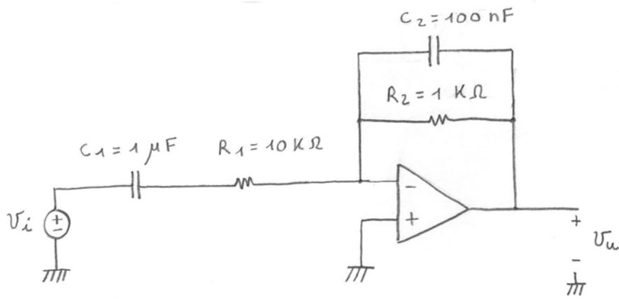
$$Z_1 = R_1 + \frac{1}{C_1 s} = \frac{1 + R_1 C_1 s}{C_1 s}$$
