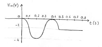
$$V_{in}(t) = \begin{cases} 2V \left[\cos\left(2\pi \frac{t}{T}\right) - 1\right] & \text{per } 0 < t < 0.5 \text{ s} \\ -2V & \text{per } t > 0.5 \text{ s} \end{cases}$$
