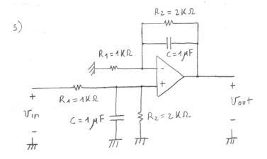
$$Z = R_2 / \frac{1}{CS} = \frac{R_2 \frac{1}{CS}}{R_2 + \frac{1}{CS}} = \frac{R_2}{1 + R_2 CS}$$
