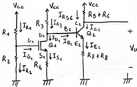
$$I_{R5C} = \frac{V_{CC} - V_U}{R_5 + R_6} = 1 \text{ mA} = I_{C2}$$
