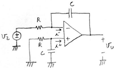
$$\text{per il c.c.v. } i^+ = 0 \rightarrow v^+ = -\left(R \parallel \frac{1}{CS}\right) i^+ = 0$$
