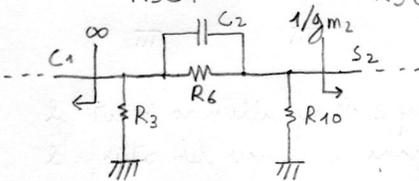
$$R_{VC2} = R_6 \parallel \left( (R_3 \parallel \infty) + (R_{10} \parallel \frac{1}{g_{m2}}) \right) = R_6 \parallel \left( R_3 + R_{10} \parallel \frac{1}{g_{m2}} \right) = 2153.267 \Omega$$
