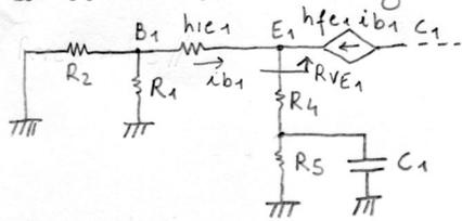
$$R_{VC1} = R_5 \parallel \left( R_4 + \frac{h_{ie1} + R_1 \parallel R_2}{h_{fe1} + 1} \right) = 1599.329 \Omega$$
